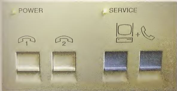
The BT Highway has not one but four separate phone sockets. Phones and faxes are plugged into sockets 1 and 2 and the terminal adaptor is plugged into one of the sockets with the blue covers.
